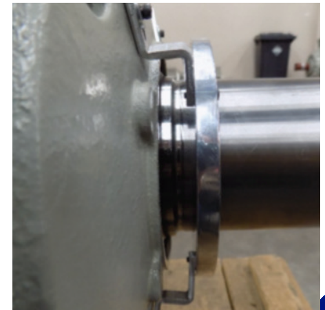
15) Use 1mm Feeler gauge to check Earthing to have a minimum of 1mm gap from the shafts shoulder, plus also check that Earthing is vertically straight at 90 degree angle / parallel with the shaft and grease cover / endshield.
