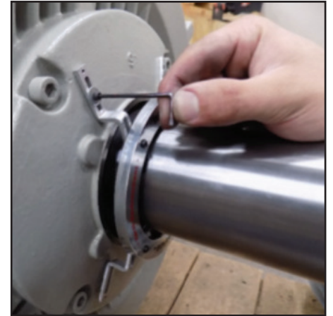
13) Fasten Earthing to grease cover /end-shield with 3mm Cap screws and 1.5mm washer. Do not tighten, leave cap screw firm but slightly loose so as to be able to allow movement of the Earthing, so as to correctly position it evenly over the shaft.
