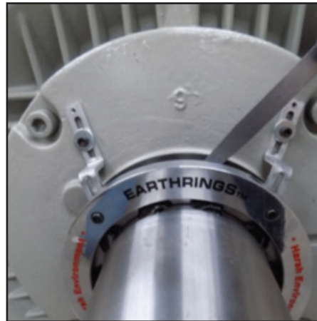
15) Use 1mm Feeler gauge to check Earthing to have a minimum of 1mm gap from the shafts shoulder, plus also check that Earthing is vertically straight at 90 degree angle / parallel with the shaft and grease cover / endshield.
