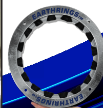
15) Use 1mm Feeler gauge to check Earthing to have a minimum of 1mm gap from the shafts shoulder, plus also check that Earthing is vertically straight at 90 degree angle / parallel with the shaft and grease cover / endshield.
