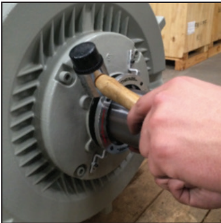
14) Move or tap Earthing so it is evenly positioned around shaft (1mm clearance over shaft), use feeler gauge 0.9mm or 0.8mm thickness to ensure even gap all around shaft.
