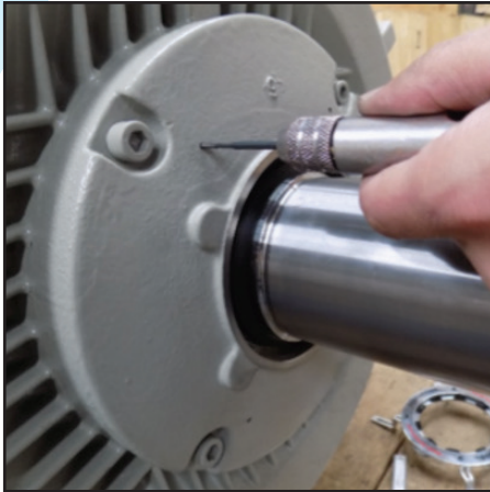
11) Tap Grease cover /endshield holes with 3mm Tap (0.5mm pitch). Use tapping fluid if required.
