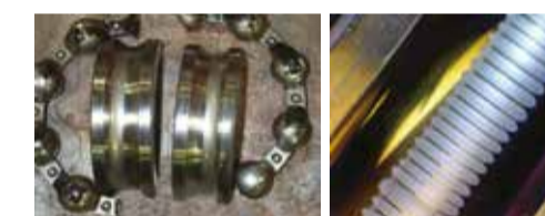
Hardening of Grease, stops Relubrication. Hardened oxidation of Grease stops new Grease entering Rollers.
