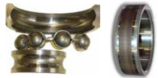
Frosted (matt) balls, frosted inner ring & fluted outer ring of ball bearing. Fluted inner ring of Roller bearing.
